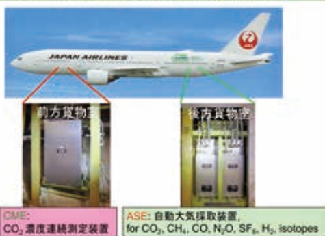
自動観測装置外観 Continuos Measuring Equipment, Automatic Sampling Equipment Outlook
